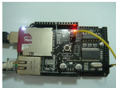
ETH_CS pin connected to Pin 53
