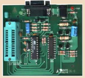
This module programs the **ATMEL AT89C2051** and **AT89C4051** microcontroller.
