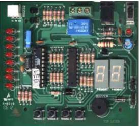
The **2051 TM-1** is a helping tool in which you can explore the many features of a microcontroller. This module uses **ATMEL AT89C2051** and **AT89C4051** microcontroller (MCU). This training module has the following applications:
